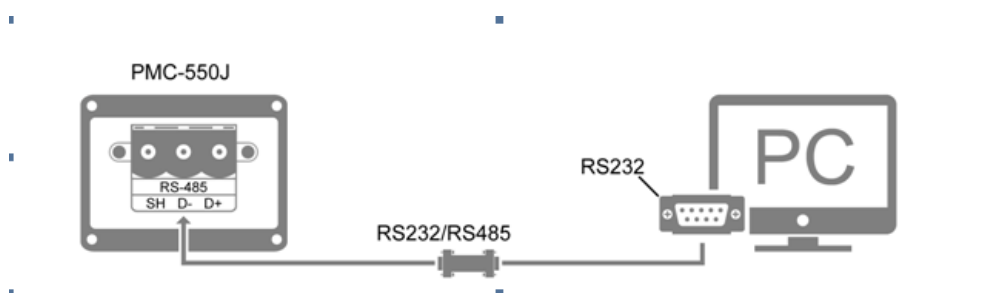
Figure 3.13 Schematic diagram of RS-485 communication wiring
