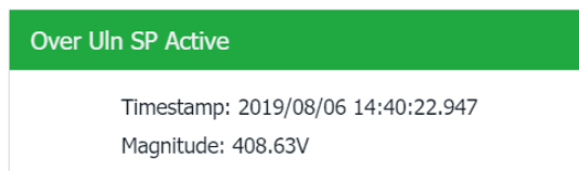
Figure 3-58 SOE Detail about Over Uln Setpoint
