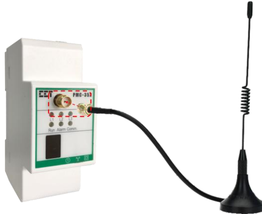
Figure 2-15 LoRa Antenna Connection
