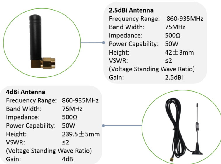
Figure 2-3 Antenna Appearances & Specifications
